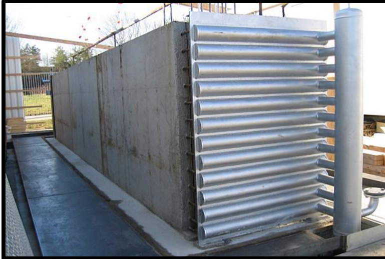
Figure 7: Un-insulated 20 m 3 Concrete Block-and-Tube TES Unit tested by Laing at DLR-German Aerospace Center (Laing et al., 2006)
