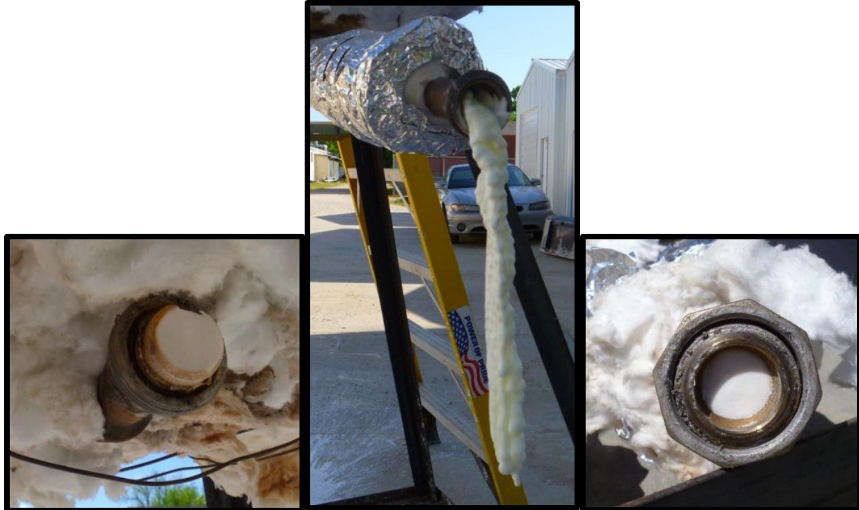
Figure 67: Salt Frozen in Lines during Testing
