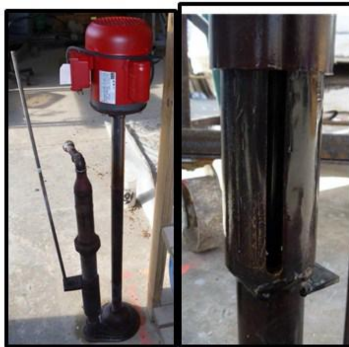
Figure 51: Salt Pumping System (Left) and Close Up of Collar and Slit (Right)
