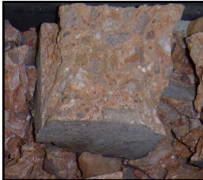
Figure 72: Crushed Mix 11 Specimen Exhibiting no Deterioration more than 1 Year After Thermal Cycling
